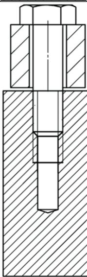
A technical drawing showing a bolt and nut assembly in a hole. The bolt is fully inserted into the hole, and the nut is being threaded onto the bolt. The hole is shown in cross-section with diagonal hatching.    |  |
